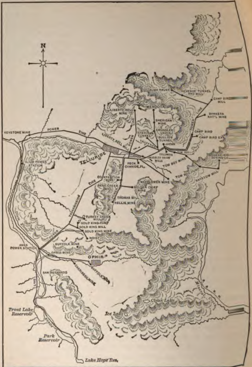
FIG. 1.—MAP OF TELLURIDE DISTRICT, SHOWING SYSTEM OF RESERVOIRS, WATERWAYS AND POWER-HOUSES, TRANSMISSION AND DISTRIBUTION LINES.
